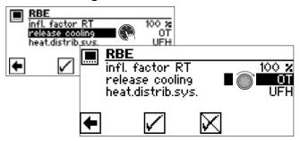
OT Releasing of cooling purely according to outdoor temperature
